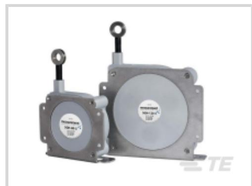
Position Sensor Product Type: **SG Series String Pots**Full Stroke Range: **2032 mm [ 80 in ]**Output Signal Type: **0 - 10 VDC, 4 - 20 mA**Accuracy: **±.35 % of FS**Repeatability: **.02 % of FS**[All String Pots 4 - 20 mA | SG Series \(2\)](#)
