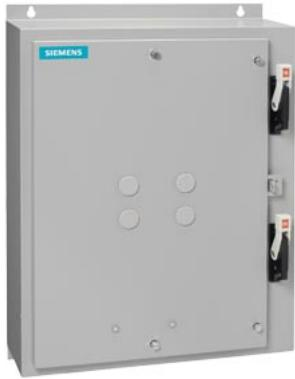
Duplex starter w/o alternator, Size 1, Three phase full voltage, Solid-state overload relay, OLR amp range 0.25-1A, 240V 50Hz / 277V 60Hz coil, Combination type, Two 3A circuit breakers, Encl NEMA type 4X 304 S-Steel, Water/dust tight noncorrosive
