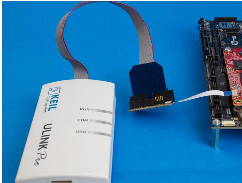
Figure 9 – ULINK Pro and debug interface board
