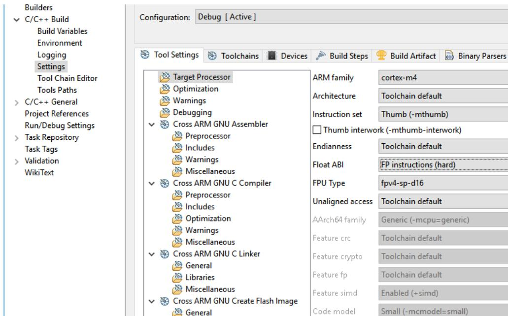
Figure 34 - Target processor
