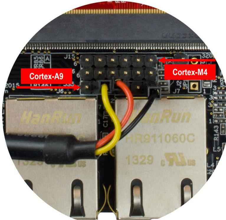
Figure 1 – COM Carrier board V1, UART connectors
