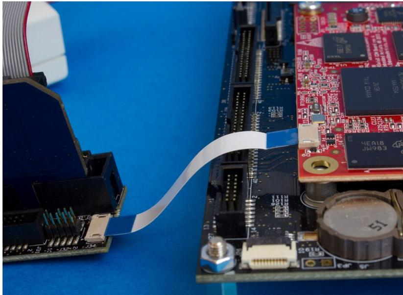
Figure 8 - Debug interface board connected to COM board
