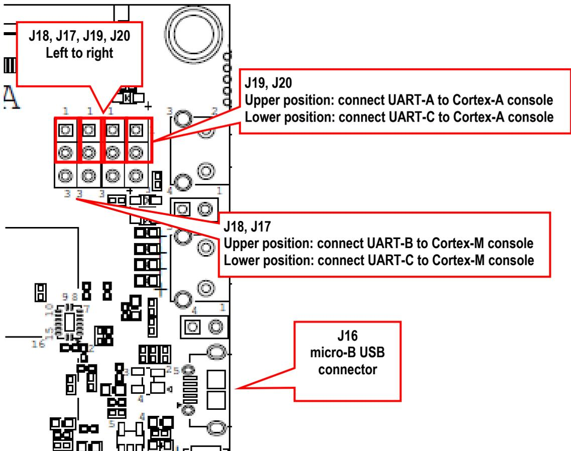
Figure 3 - COM Carrier board V2, UART interface connectors
