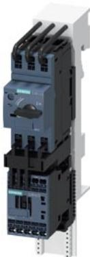
Load feeder fuseless, Direct-on-line starting 400 V AC, Size S00 1.10...1.60 A 24 V DC Spring-type terminal for 60 mm busbar systems (also fulfills type of coordination 1) Type of coordination 2,  $I_q = 150 \text{ kA}$  1 NO (contactor)
