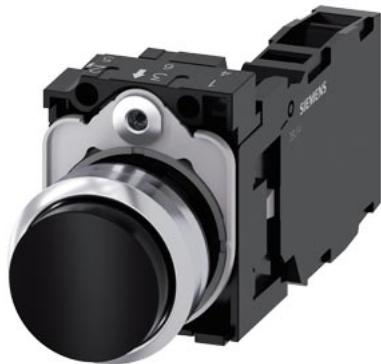
Pushbutton, 22 mm, round, metal, shiny, black, pushbutton, raised, momentary contact type, with holder, 1 NO+1 NC, screw terminal, with laser labeling, upper case and lower case, always upper case at the beginning of the word
