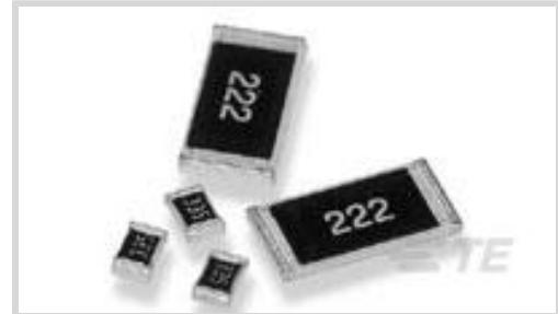
Resistor Type: **Power Resistor**Element Type: **Thick Film**Package Size Code: **0603**Power Rating: **.2 W**Resistance Value: **560 Ω**
