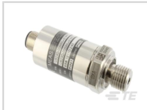
Pressure Sensor Type: **Industrial Pressure Transducer**Pressure: **2.068 bar [ 30 psi ]**Pressure Type: **Absolute**Supply Voltage Range: **8 - 30 V**Output Signal Type: **1 - 5 V**
