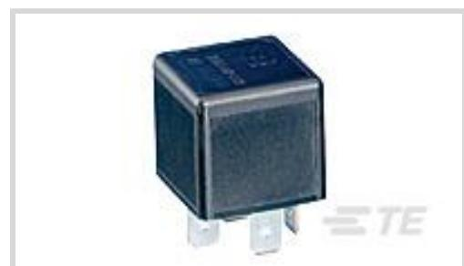
Coil Voltage Rating: **12 VDC**Contact Current Class: **30 - 50 A**Contact Arrangement: **1 Form C (CO)**Product Mount Type: **Socket**Coil Resistance: **90 Ω****Features****Configuration Features**
