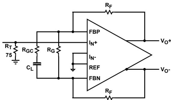
$$\text{DC Gain} = 1 + \frac{2R_F}{R_G}$$
