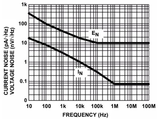
FIGURE 10. VOLTAGE AND CURRENT NOISE vs FREQUENCY
