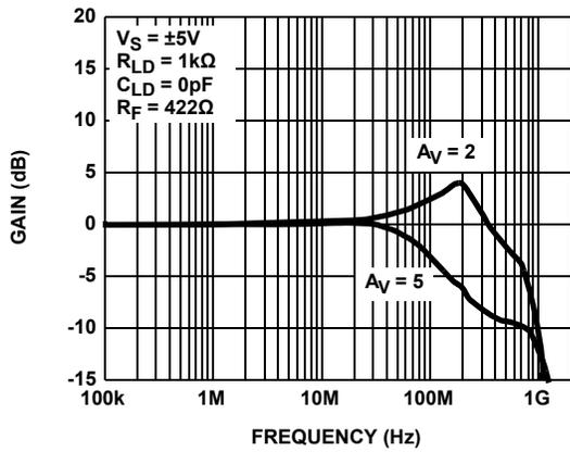
FIGURE 7. EL5378 FREQUENCY RESPONSE FOR VARIOUS GAIN
