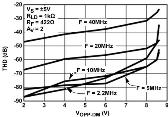
FIGURE 17. TOTAL HARMONIC DISTORTION vs DIFFERENTIAL OUTPUT SWING
