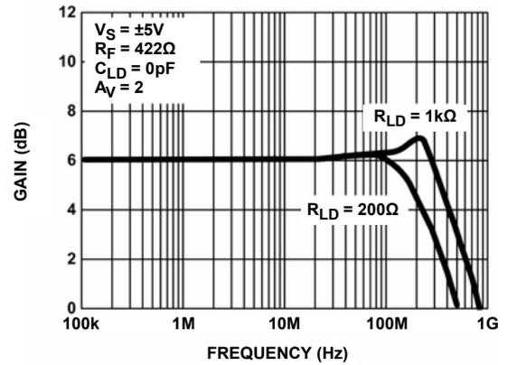
FIGURE 4. EL5178 FREQUENCY RESPONSE FOR VARIOUS  $R_{LD}$
