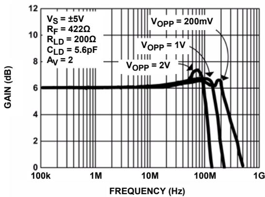
FIGURE 5. EL5178 FREQUENCY RESPONSE FOR VARIOUS  $V_{OPP}$
