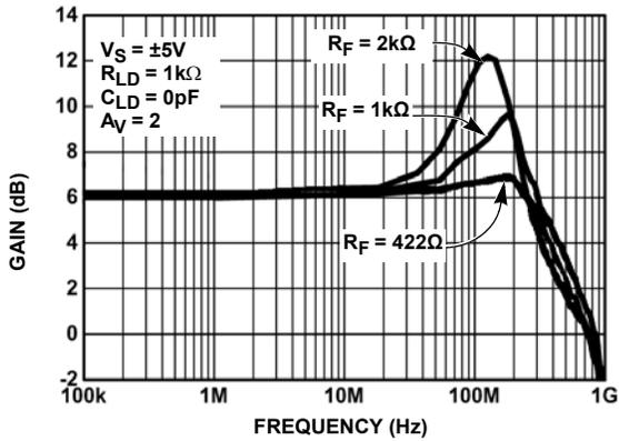
FIGURE 1. EL5178 FREQUENCY RESPONSE FOR VARIOUS  $R_f$
