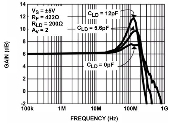
FIGURE 8. EL5378 FREQUENCY RESPONSE FOR VARIOUS  $C_{LD}$
