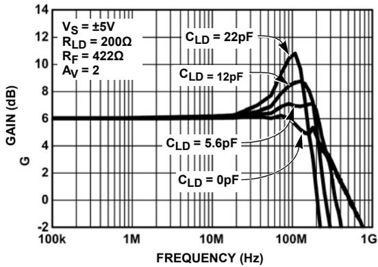
FIGURE 3. EL5178 FREQUENCY RESPONSE FOR VARIOUS  $C_{LD}$
