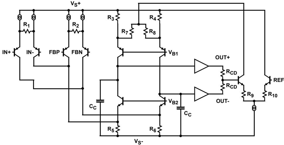
FIGURE 34. SIMPLIFIED SCHEMATIC
