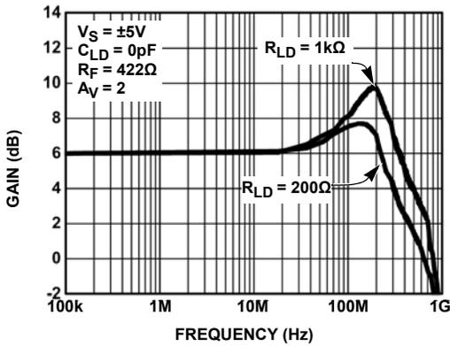
FIGURE 9. EL5378 FREQUENCY RESPONSE FOR VARIOUS  $R_{LD}$
