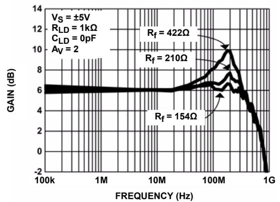
FIGURE 6. EL5378 FREQUENCY RESPONSE FOR VARIOUS  $R_f$
