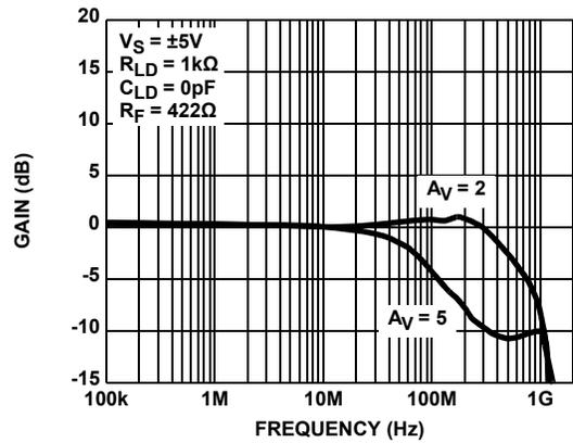
FIGURE 2. EL5178 FREQUENCY RESPONSE FOR VARIOUS GAIN
