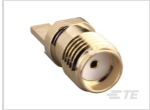
RF Interface: **SMA**RF Connector Style: **Jack**Impedance: **50 Ω**RF Connector Coupling Mechanism: **Threaded**Operating Frequency: **0 - 26.5 GHz**
