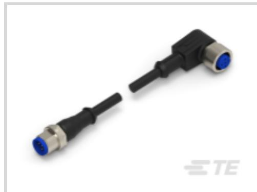
M8/M12 Application Type: **Sensor/Actuator**Number of Positions: **5**Connector & Keying Code: **A**Connector Type (End A): **M12 Plug**Connector Type (End B): **M12 Socket**[All M12 MS-FR Double End Cable Assembly BL \(9\)](#)
