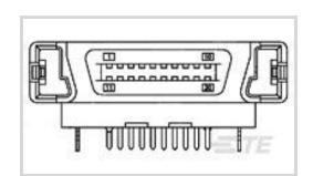
PCB Connector Assembly Type: PCB Mount Receptacle
