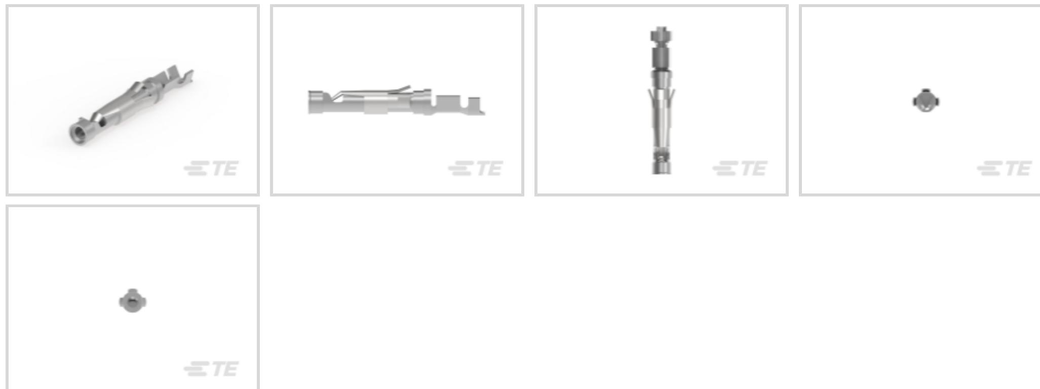
Contact Type: **Socket**Contact Mating Area Plating Material: **Tin**Wire Contact Termination Area Plating Material: **Tin**Contact Size: **Size 16**Wire Size: **24 - 20 AWG**
