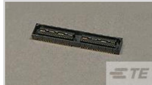
PCB Connector Assembly Type: **PCB Mount Receptacle**PCB Mount Orientation: **Vertical**Connector System: **Board-to-Board**Number of Positions: **80**Centerline (Pitch): **.8 mm [.031 in]**
