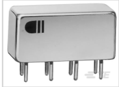
Contact Arrangement: **2 Form C, DPDT, 2 C/O**Input Voltage: **26.5 VDC**Contact Current Rating: **2 A**Coil Voltage Rating: **26.5 VDC**Coil Resistance: **1350 Ω**[All DPDT Relay:Electrically-Held, 1/5-Size Relay \(84\)](#)
