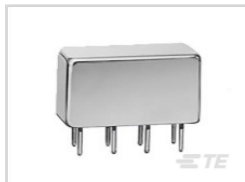
Contact Arrangement: **2 Form C, DPDT, 2 C/O**Input Voltage: **26.5 VDC**Contact Current Rating: **5 A**Coil Voltage Rating: **26.5 VDC**Coil Resistance: **700 Ω**
