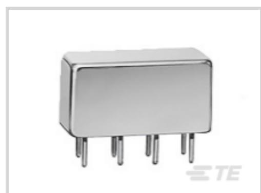
Contact Arrangement: **2 Form C, DPDT, 2 C/O**Input Voltage: **26.5 VDC**Contact Current Rating: **2 A**Coil Voltage Rating: **26.5 VDC**Coil Resistance: **700 Ω**
