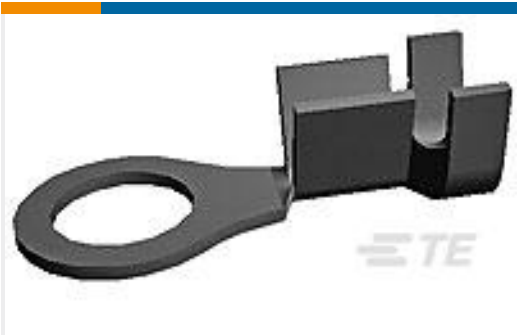
TE Part # 280268-2 RING TONGUE 4-6MM2 0.0276X0.650 TPBR
