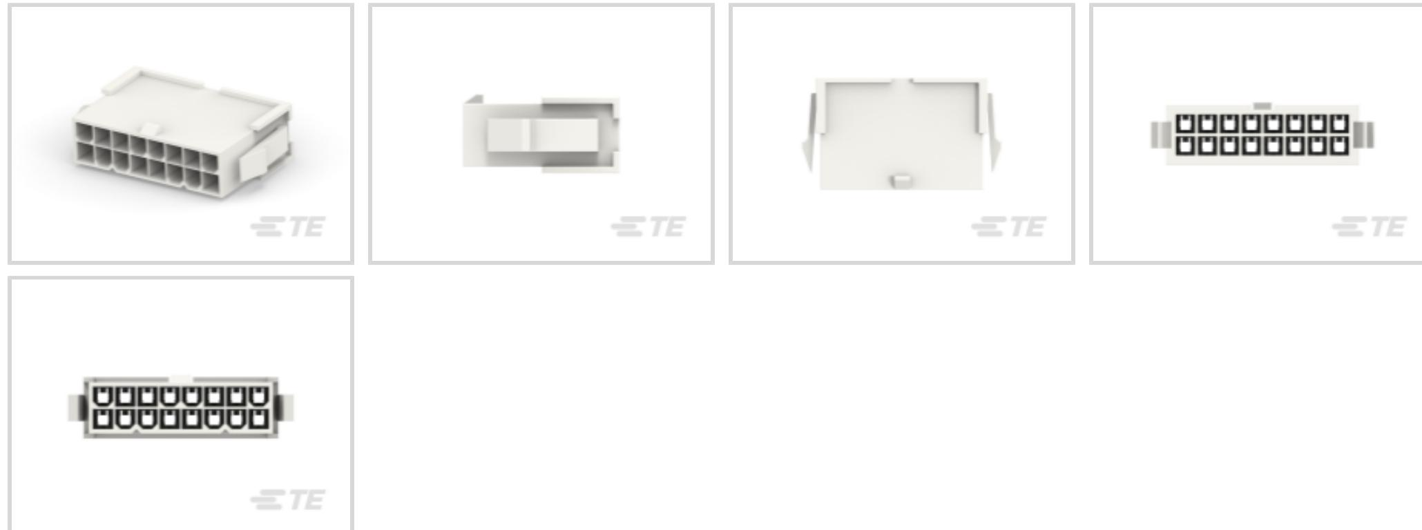
Rectangular Power Connector Type: **Housing**Connector & Housing Type: **Plug**Connector System: **Wire-to-Panel, Wire-to-Wire**Number of Positions: **16**Centerline (Pitch): **4.2 mm [.165 in]**
