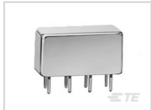
Contact Arrangement: **2 Form C, DPDT, 2 C/O**Input Voltage: **26.5 - 32 VDC**Contact Current Rating: **2 A**Coil Voltage Rating: **32 VDC**Coil Resistance: **1250 Ω**
