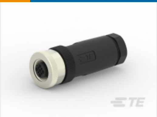
TE Part # T4110002051-000 M12,FEMALE,STRAIGHT,A CODE,5P, PG9,GOLD
