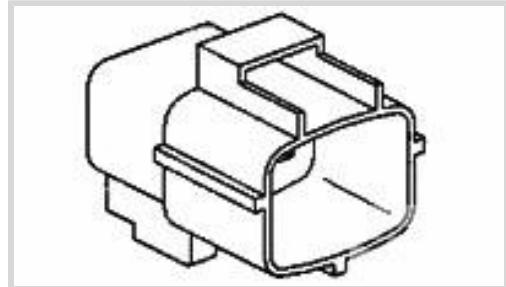
Connector System: **Wire-to-Wire**
