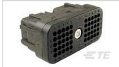
Connector System: **Wire-to-Wire**Number of Positions: **50**Connector & Housing Type: **Housing for Female Terminals**Centerline (Pitch): **4.42 mm [ .174 in ]**Sealable: **Yes**[All DEUTSCH DRC Housings \(117\)](#)
