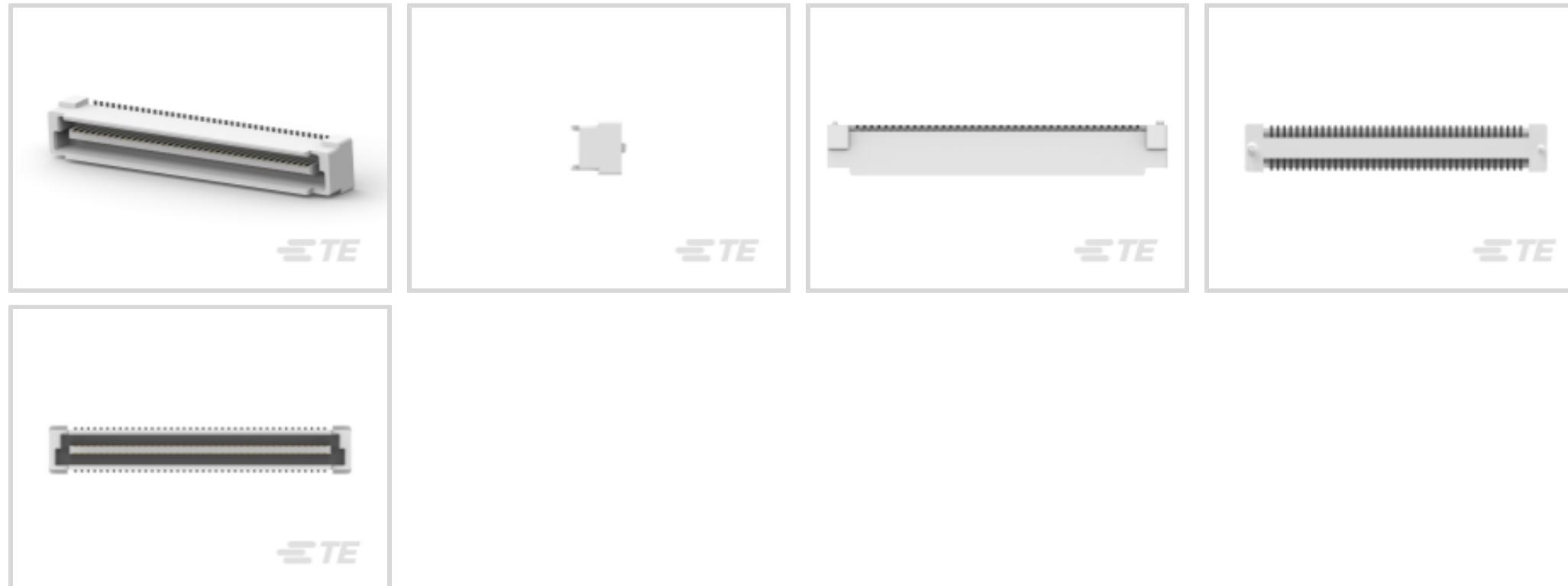
PCB Connector Assembly Type: **PCB Mount Header**PCB Mount Orientation: **Vertical**Connector System: **Board-to-Board**Number of Positions: **80**Centerline (Pitch): **.8 mm [.031 in]**[All Free Height Plug Connector: Board-Board, Vertical, 80, 0.8mm \(18\)](#)**Features****Product Type Features**
