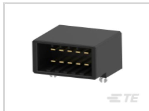
Connector System: **Wire-to-Board**Number of Positions: **10**Number of Rows: **2**Centerline (Pitch): **3.81 mm [.15 in]**PCB Mount Orientation: **Horizontal****All Header Assembly: Wire-to-Board, 15A, gold or tin plated (120)**
