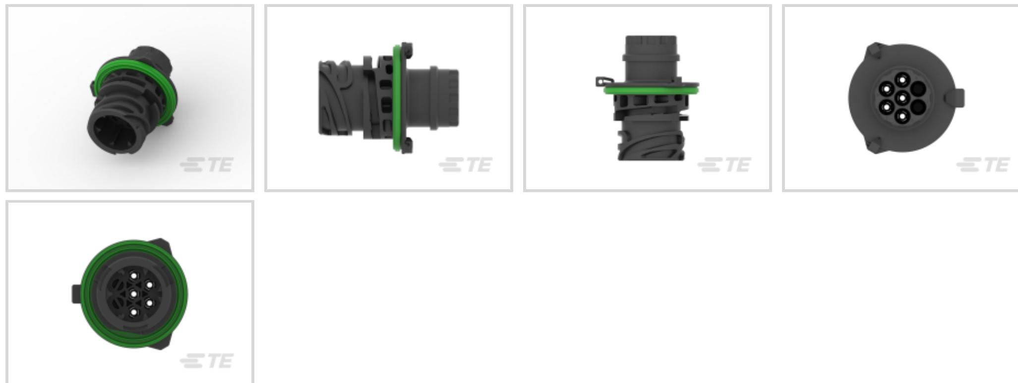
Connector System: **Wire-to-Wire**Number of Positions: **5**Connector & Housing Type: **Housing for Male Terminals**Centerline (Pitch): **11.4 mm [.449 in]**Sealable: **Yes**[All Circular DIN Housings \(59\)](#)
