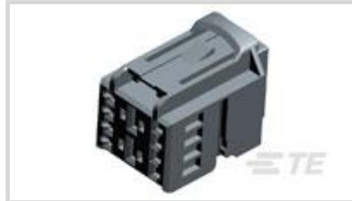
Connector System: **Wire-to-Board, Wire-to-Wire**Number of Positions: **10**Connector & Housing Type: **Housing for Female Terminals**Centerline (Pitch): **2.54 mm, 5.2 mm [ .1 in, .205 in ]**Sealable: **No**
