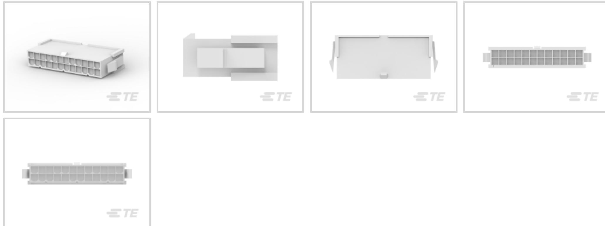
Rectangular Power Connector Type: **Housing**Connector & Housing Type: **Plug**Connector System: **Wire-to-Panel, Wire-to-Wire**Number of Positions: **24**Centerline (Pitch): **4.2 mm [.165 in]**
