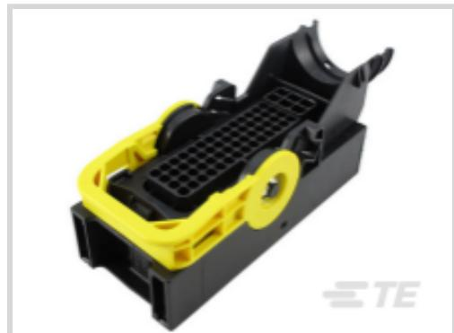
Connector System: **Wire-to-Board, Wire-to-Device, Wire-to-Wire**Number of Positions: **62**Connector & Housing Type: **Housing for Female Terminals**Centerline (Pitch): **4 mm, 5 mm [ .157 in, .197 in ]**Sealable: **Yes**[All LEAVYSEAL Housings \(64\)](#)
