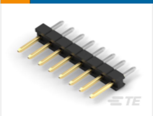
TE Part # 1-2355172-0 10P, 2MM, BRK HDR, SRVT, 2, 8, 0.1AU, BOX
