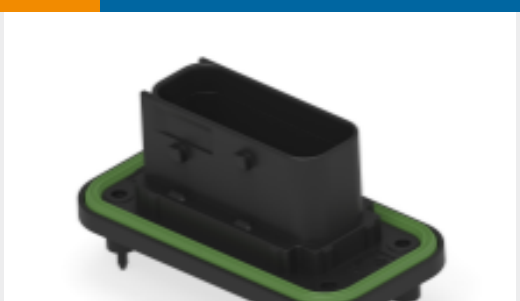
TE Part # 1-2377481-1 18POS,TAB1.5X0.64,HDR ASSY, 180DEG,COD A
