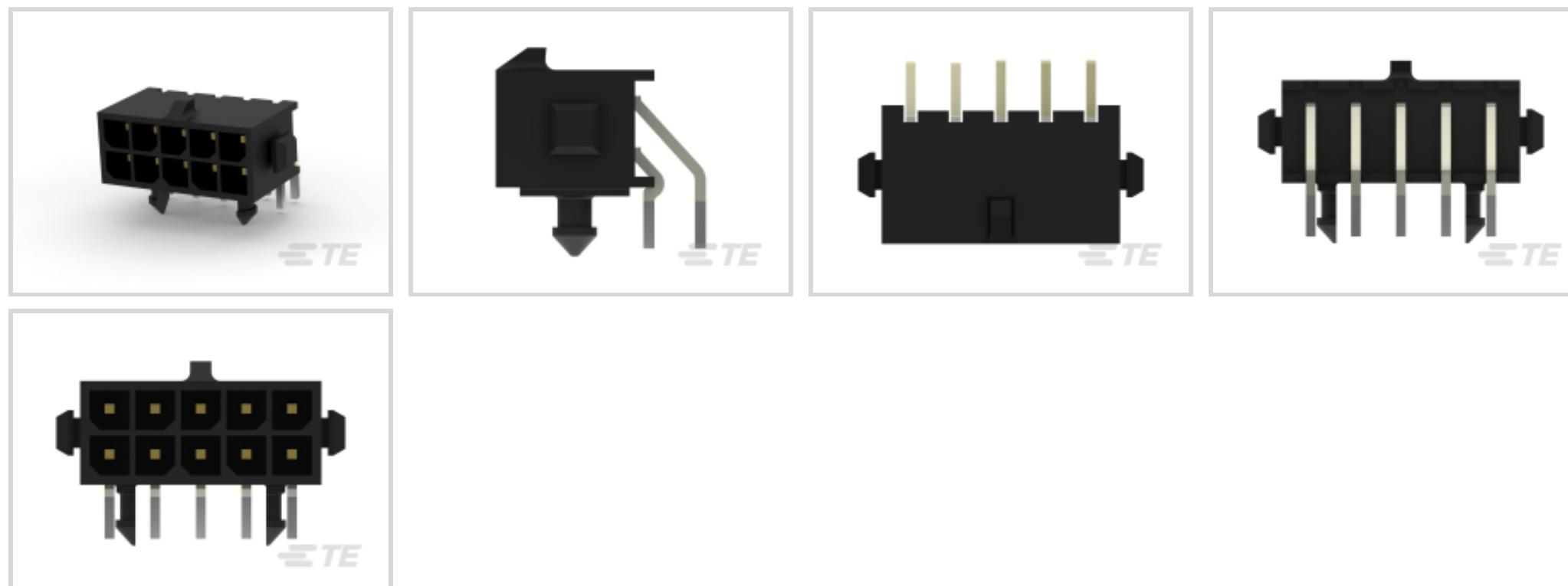
Rectangular Power Connector Type: **Header**Connector & Housing Type: **Plug**Connector System: **Wire-to-Board**Number of Positions: **10**Centerline (Pitch): **3 mm [.118 in]****Features****Product Type Features**
