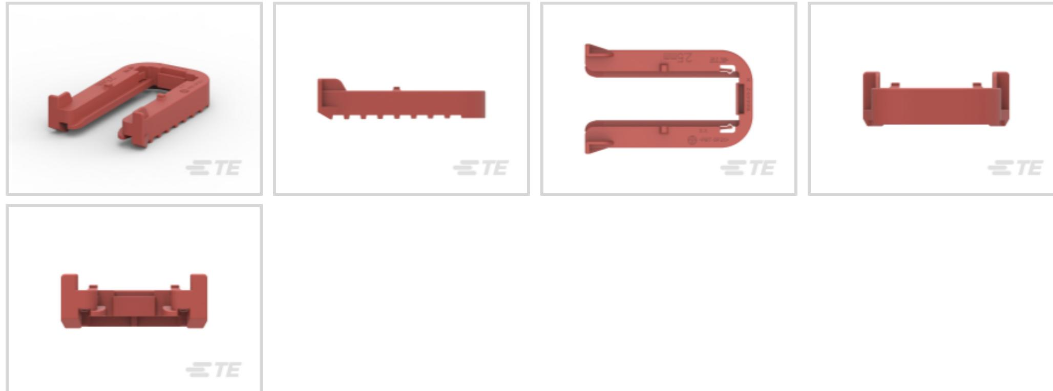
Automotive Connector Accessory Type: **Mounting Clip**Primary Product Material: **PBT GF**Primary Product Color: **Red**Operating Temperature Range: **-40 - 140 °C [-40 - 284 °F]**[All Heavy Duty Sealed Connector Series Fixing Slides \(33\)](#)
