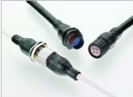
CeeLok FAS-T connectors offer a small form factor, field terminable I/O connector capable of 10 Gb/s Ethernet. Crimp-snap contacts enable easy termination and field repairability. The integral backshell offers easy 360-degree shield termination.
