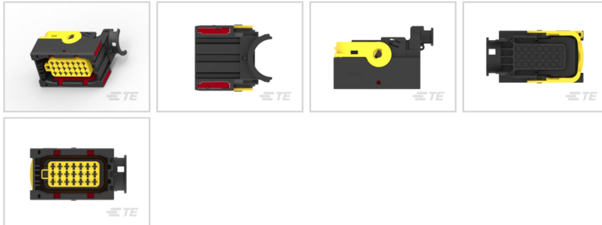
Connector System: **Wire-to-Board, Wire-to-Device, Wire-to-Wire**Number of Positions: **21**Connector & Housing Type: **Housing for Female Terminals**Centerline (Pitch): **5.5 mm [.197 in]**Sealable: **Yes**[All LEAVYSEAL Housings \(64\)](#)
