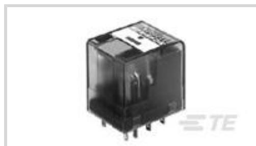
Relay Type: **Industrial Panel Plug-In**Coil Magnetic System: **Monostable**Coil Power Rating DC: **750 mW**Coil Resistance: **20833 Ω**Coil Special Features: **UL Coil Insulation Class F**
