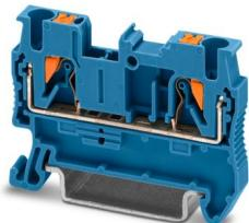
Feed-through terminal block, nom. voltage: 800 V, nominal current: 24 A, number of connections: 2, number of positions: 1, connection method: Push-in connection, Rated cross section: 2.5 mm<sup>2</sup>, cross section: 0.14 mm<sup>2</sup> - 4 mm<sup>2</sup>, mounting type: NS 35/7,5, NS 35/15, color: blue
