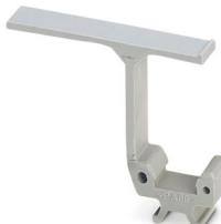
Group marking label, can be snapped into terminal center for screw, spring-cage, push-in, and fast connection terminal blocks, can be labeled with a 24 x 4 mm label or manually using B-STIFT, in the foot part with ZB 5
