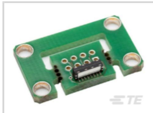
Position Sensor Product Type: **Magnetic Linear Position Sensor**Sensor Package: **DFN2x6**Sensing Range: **5 mm**Output Signal Type: **Passive Analog**Typical Signal Amplitude: **11 mV/V**[All AMR Position Sensors \(6\)](#)
