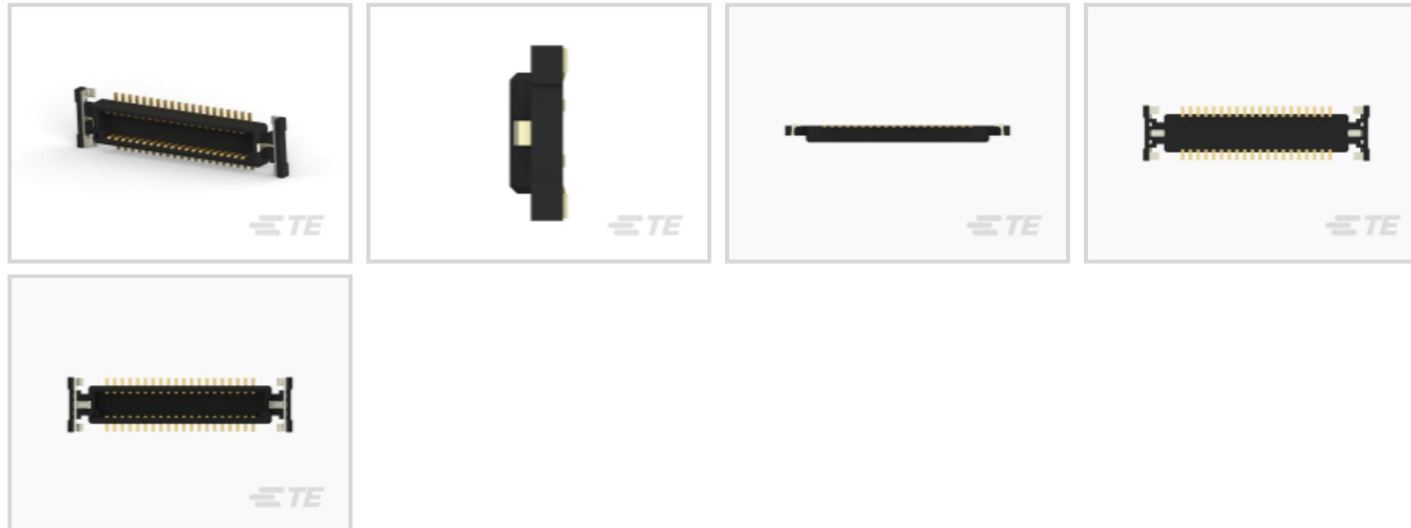
PCB Connector Assembly Type: **PCB Mount Header**PCB Mount Orientation: **Vertical**Connector System: **Board-to-Board**Number of Positions: **40**Centerline (Pitch): **.5 mm [ .02 in ]**
