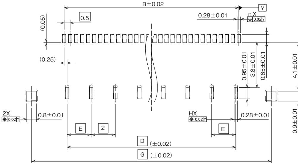
Recommended PCB Mounting Thickness : 0.12
