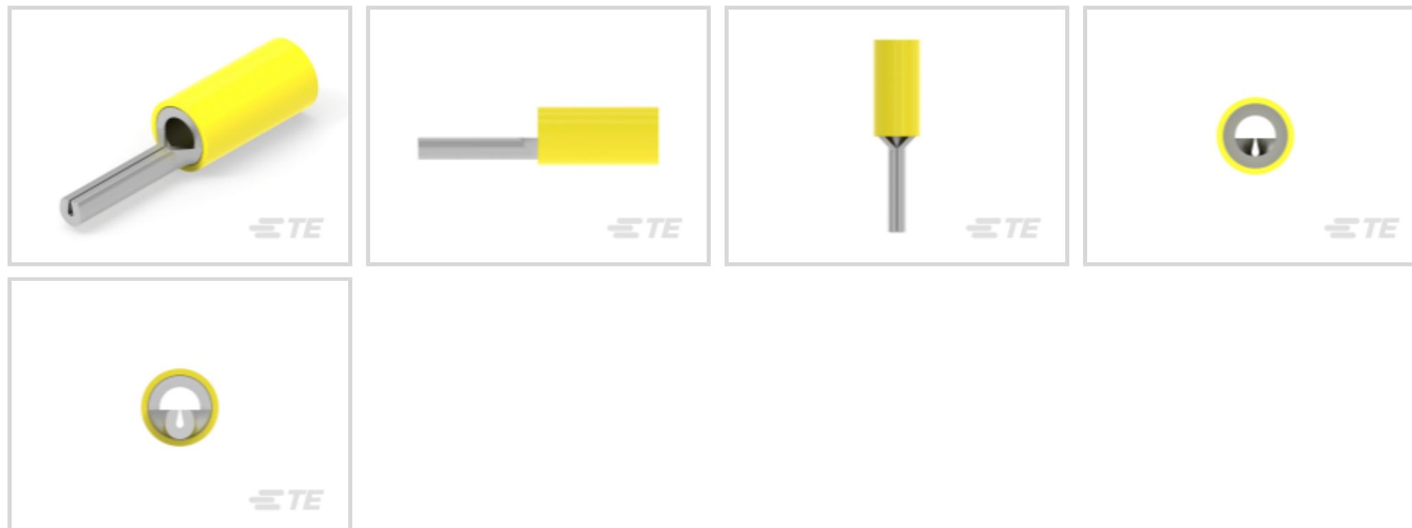
Crimp Wire Terminal Type: **Wire Pin**Mating Pin Diameter: **2.6 mm [.102 in]**Compatible Insulation Diameter Range: **3.81 - 6.35 mm, 6.4 mm [.15 - .25 in, .251 in]**Wire Size: **3 - 6 mm<sup>2</sup>**
