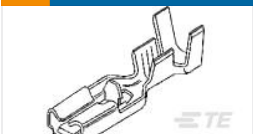
TE Part # 63407-2 PL 187 TERMINAL REC 0.2-0.5 MM2 PTPBR
