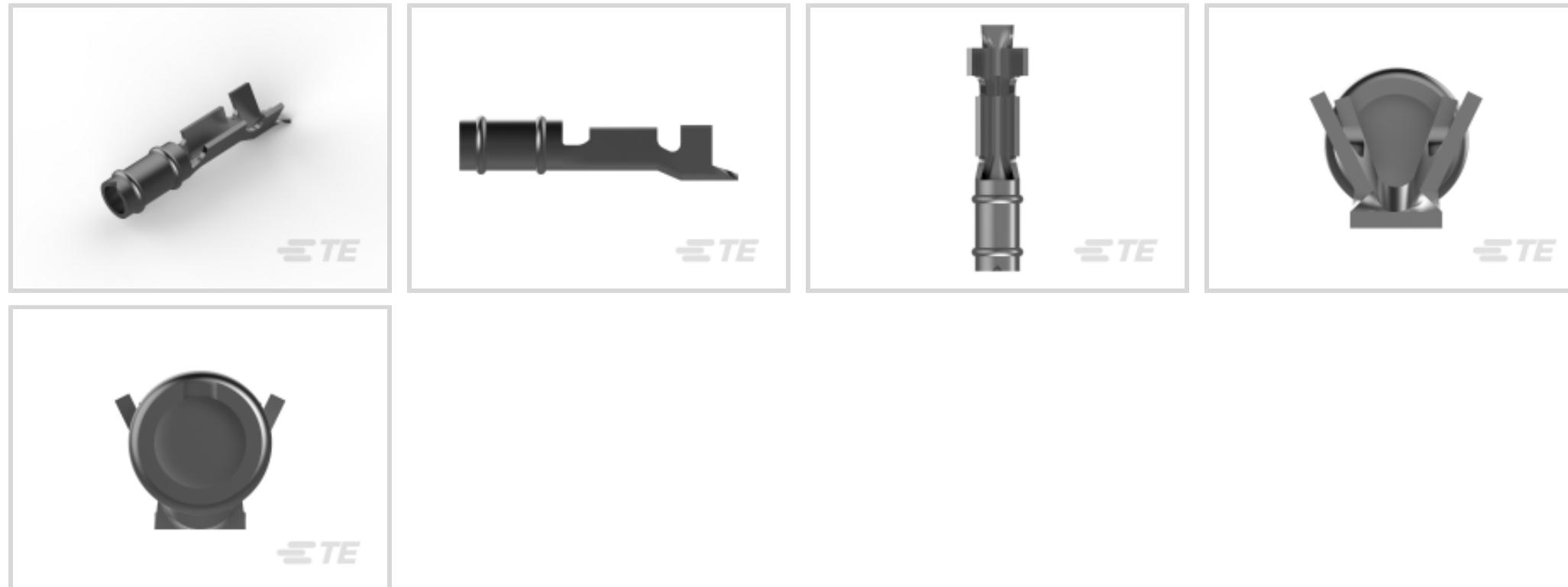
PCB Terminal Type: **Receptacle**PCB Hole Diameter: **3.18 mm [.125 in]**Mating Pin Diameter: **1.47 mm [.058 in]**Compatible Insulation Diameter (Max): **1.65 mm [.065 in]**Compatible Insulation Diameter Range: **.89 – 1.65 mm [.035 – .065 in]****Features****Product Type Features**
