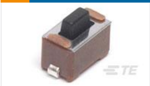
TE Part # 147873-2 SWITCH,TACT,SMT,J-LEAD,4.3MM
