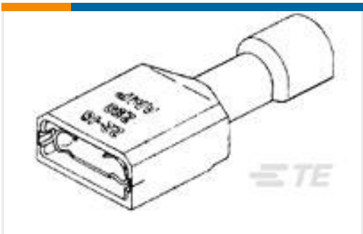
TE Part # 2-520193-2 ULTRA-FAST 187 ASY REC 22-18 TPBR
