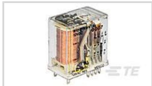
Relay Type: **Industrial Panel Plug-In**Coil Magnetic System: **Monostable**Coil Power Rating DC: **1400 mW**Coil Resistance: **430 Ω**Coil Special Features: **Sensitive Version**
