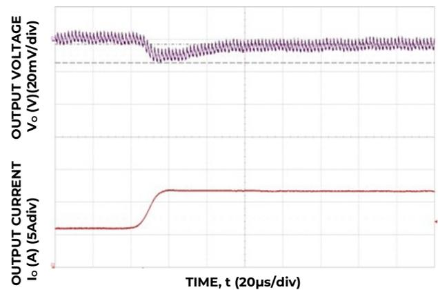
Figure 4. Transient Response to Dynamic Load Change from 50% to 100% on one output at 12V<sub>in</sub>,  $C_{out} = 2 \times 47\mu\text{F} + 7 \times 330\mu\text{F}$ ,  $C_{Tune} = 12\text{nF}$ ,  $R_{Tune} = 300\Omega$
