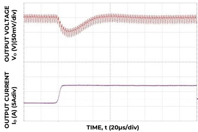
Figure 22. Transient Response to Dynamic Load Change on one output from 50% to 100% at 12V<sub>in</sub>,  $C_{out} = 3 \times 47\mu\text{F} + 2 \times 330\mu\text{F}$ ,  $C_{Tune} = 1500\text{pF}$  &  $R_{Tune} = 300\Omega$
