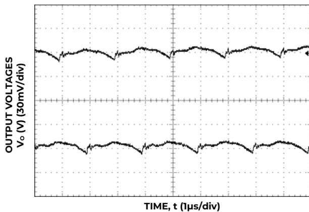
Figure 3. Typical output ripple and noise ( $C_o = 2 \times 0.1\mu\text{F} + 2 \times 47\mu\text{F}$  ceramic,  $V_{IN} = 12\text{V}$ ,  $I_o = I_{o1,max}, I_{o2,max}$ ).
