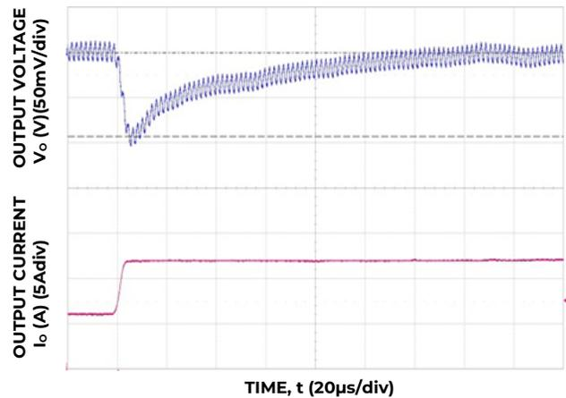
Figure 34. Transient Response to Dynamic Load Change on one output from 50% to 100% at 12V<sub>in</sub>,  $C_{out} = 6 \times 47\mu F$ ,  $C_{Tune} = 470pF$  &  $R_{Tune} = 300\Omega$
