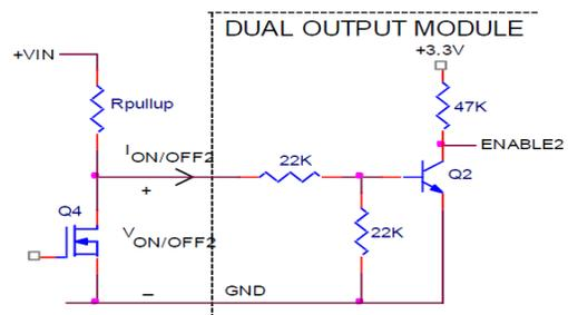
Figure 40. Circuit configuration for using negative On/Off logic.
