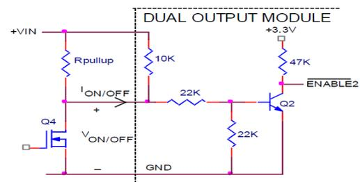
Figure 39. Circuit configuration for using positive On/Off logic.
