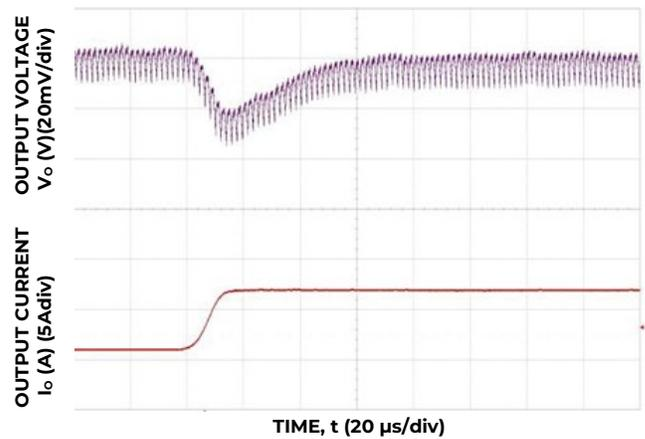
Figure 10. Transient Response to Dynamic Load Change on one output from 50% to 100% at 12V<sub>in</sub>,  $C_{out} = 3 \times 47\mu\text{F} + 3 \times 330\mu\text{F}$ ,  $C_{Tune} = 2700\text{pF}$  &  $R_{Tune} = 300\Omega$
