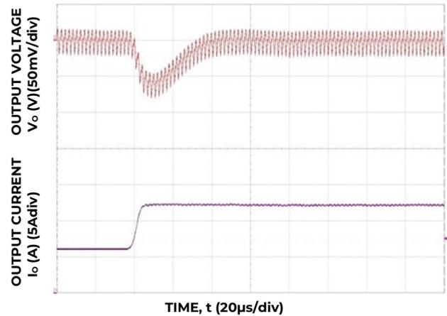
Figure 28. Transient Response to Dynamic Load Change on one output from 50% to 100% at 12V<sub>in</sub>,  $C_{out} = 3 \times 47\mu F + 1 \times 330\mu F$ ,  $C_{Tune} = 1200pF$  &  $R_{Tune} = 300\Omega$
