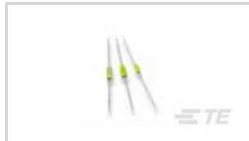
Inductor Type: **Radio Frequency**Inductance: **10  $\mu$ H**Current Rating (Max): **219 mA**DC Resistance: **3.7  $\Omega$** Inductor Quality Factor: **55**
