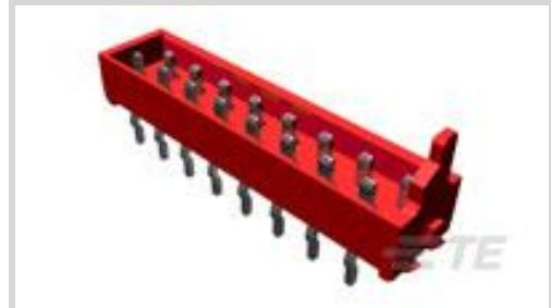
Connector System: **Board-to-Board**Number of Positions: **16**Centerline (Pitch): **1.27 mm [.05 in]**PCB Mount Retention: **With**PCB Mount Retention Type: **Kinked Solder Tails**[All Male-on-Board Connector, Micro-MaTch \(36\)](#)
