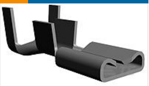
TE Part # 63596-2 187 FASTON REC 18-14 AWG TPBR
